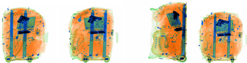
Figure 5: Four views generated during a scan. The Y-axis is the conveying direction. Images scanned with a laboratory prototype not in TSA configuration.
